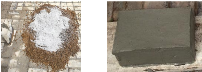
Figure 2- Mixing and casted brick
